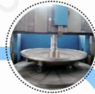
Processing cylinder head
