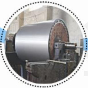
Fine grinding cylinder surface
