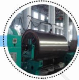
Fine turning dryer cylinder
