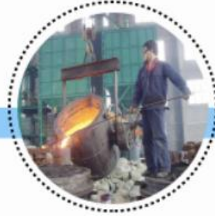
Pouring cylinder head
