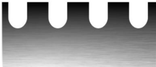
Grooved cast iron dryer shell
