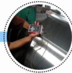
Surface hardness test
