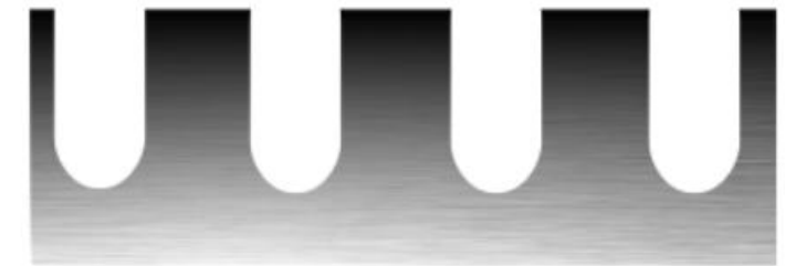
Grooved steel dryer shell
